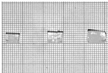
2.2 Figure 1. Photograph of BTSN-Kcl crystals
