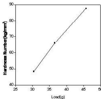
Figure 6. Variation of hardness with load for BTSN-KCl crystal
