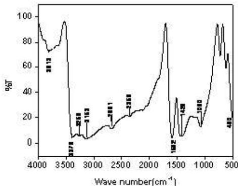
Figure 5. FTIR Spectrum of BTSN-KCl
